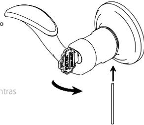
Rotate key counterclockwise 90° while pressing wire into hole.
