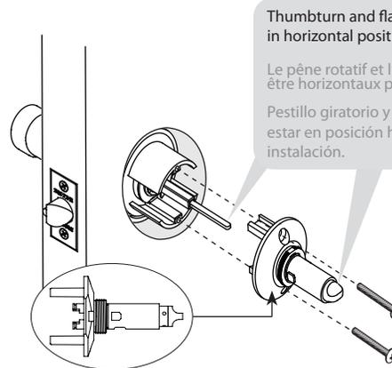
Thumbturn and flat spindle **MUST** be in horizontal position for installation
