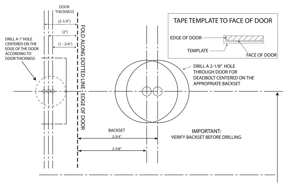
LOCATE CENTERLINE FOR HOLE APPROXIMATELY 36"TO 38"FROM FLOOR
